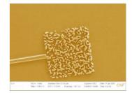
Integrated Disordered Optical Resonators, CNF Project # 980-01. PI: Michal Lipson, Electrical and Computer Engineering, Cornell University, mlipson@ece.cornell.edu. Figure: SEM of disordered resonator in SOI.
