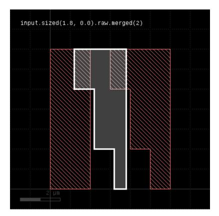
The "merged" method with an argument of 2 will produce output where more than two polygons overlap. The size function by default creates a clean layer, but separate polygons for each input polygon, so by using "raw", the layer is switched into raw mode that makes the individual polygons accessible without merging them into one bigger polygon.
